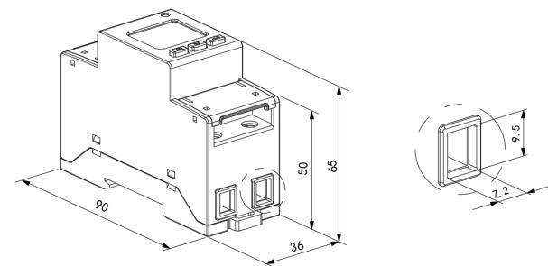
Note: The torque of direct connect should not be greater than 4.0N·m.
